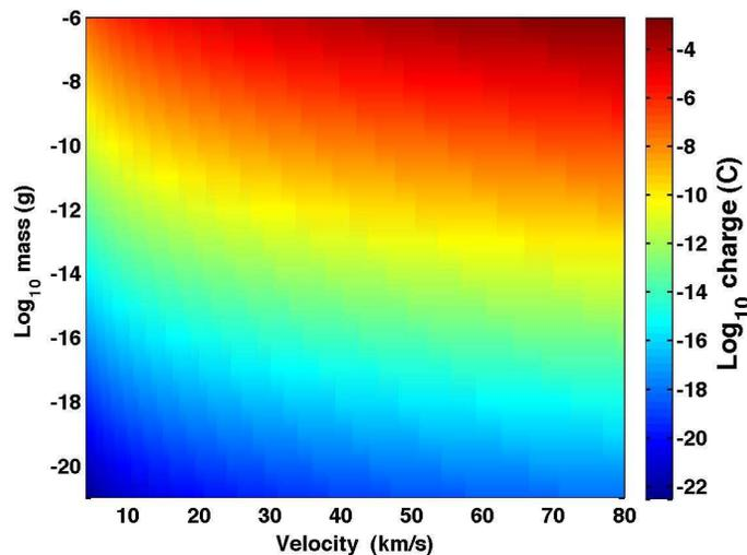
Figure 1. Charge (in coulombs) produced by a particle after impact with a spacecraft, as a function of particle mass and velocity.
