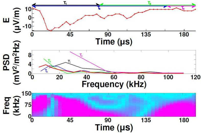
**Figure 5. Waveform, discrete Fourier analysis and wavelet analysis associated with impacts from nanometer-sized particles at solar wind velocity (450 km/s), as detected by Cassini’s RPWS dipole antennas.**
