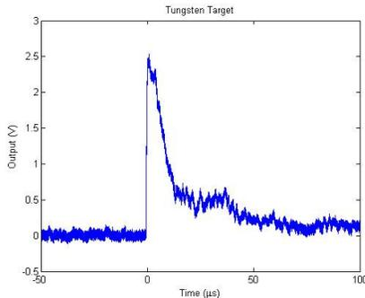
**Figure 6 Typical response of the photomultiplier tube to the flash from a hypervelocity impact observed during ground based testing in August 2011**
