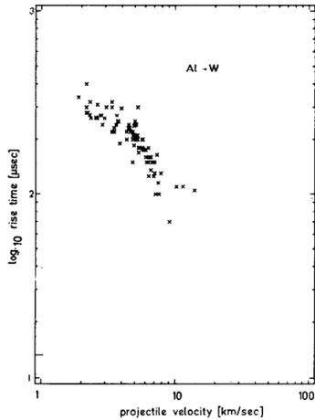
**Figure 7 Variation of rise time of integrated signal with projectile velocity [9]**
