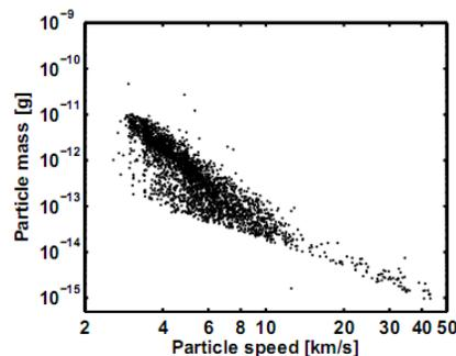
**Figure 2 Distribution of projectile masses and speeds during first round of testing at MPIK in December 2010**
