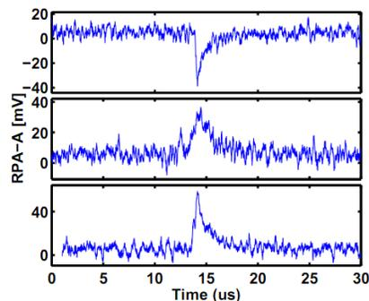
**Figure 5** Signals from impacts on negatively charged (top panel), uncharged (middle panel) and positively charged (bottom panel) Tungsten target. The projectile speeds for these impacts were 4.7km/s, 3.0km/s and 3.1km/s and projectile masses were 2.2pg, 7.2pg and 8.9pg respectively.
