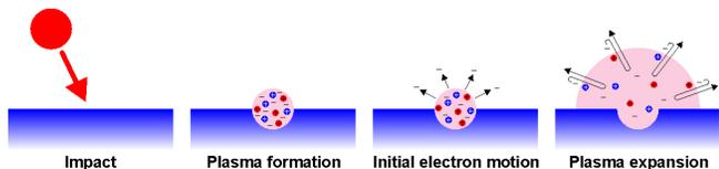
**Figure 1 An illustration of the plasma generation and expansion process following a hypervelocity impact**
