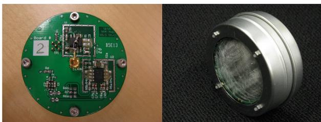
**Figure 4** Images of the Retarding Potential Analyzer. The transimpedance amplifier board is on the left and the fully-assembled sensor is on the right
