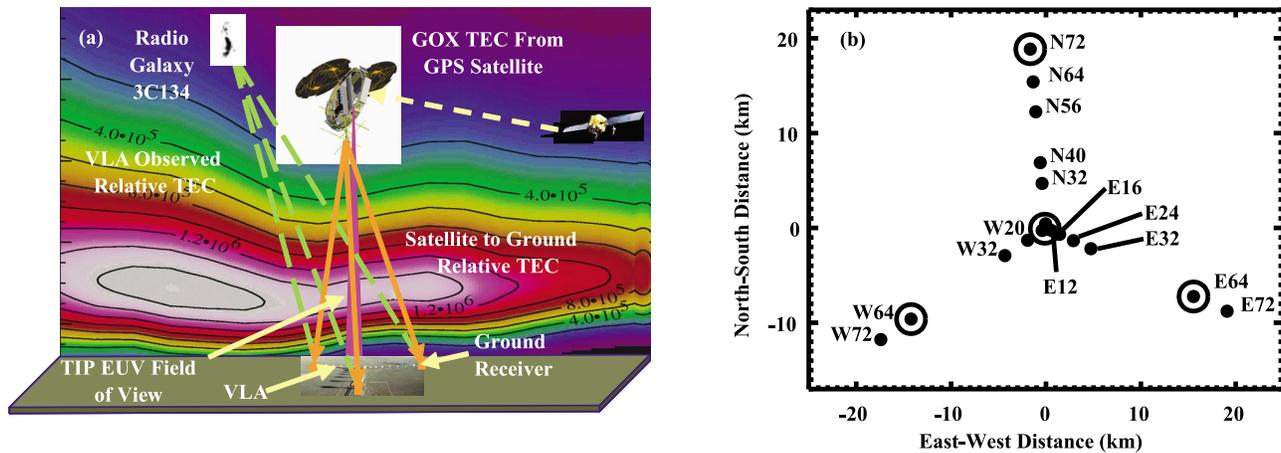
**Figure 1.** CRICKET Concept. (a) The experiment concept. (b) The VLA in the A-configuration. The antennas used in the campaign are indicated, with circles indicating the antennas with co-located TBB receivers. The antennas nearest the center of the array overlap in this figure and hence are not visible.
